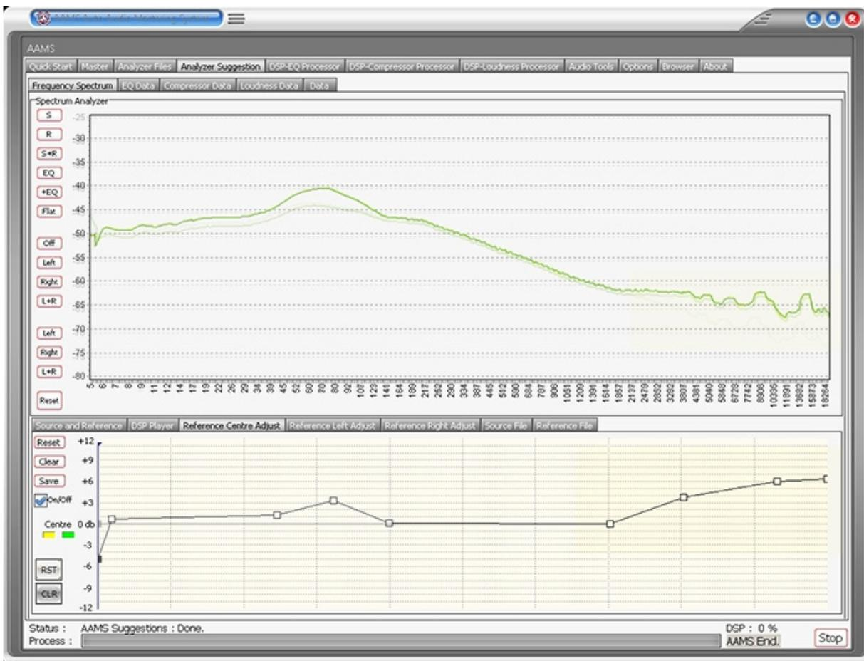
For more adjusting, we have created some extra bass frequencies in the spectrum around 80 hz and have a little cutoff in the beginning at 5-20 hz.
